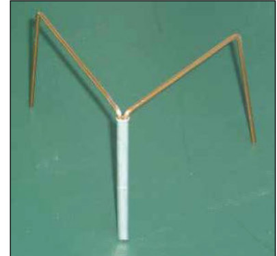
This frame uses a small metal tube to provide the hinge for the frames
