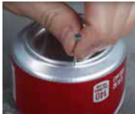
With a small nail punch a collection of holes equally placed around the rim
