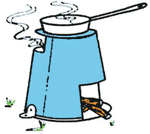
Very simple rocket stove using a metal bucket
