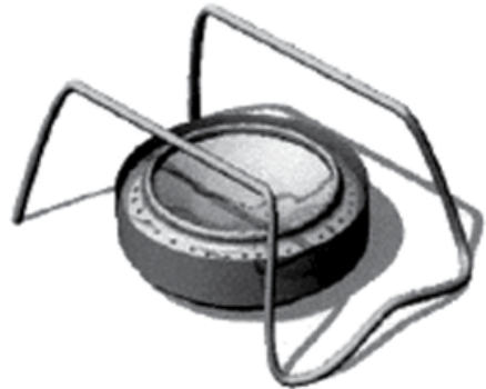
Two wire frames joined by a simple wire joint that allows the frame to be folded flat.
