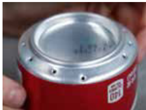
With a small nail punch a collection of holes equally placed around the rim
