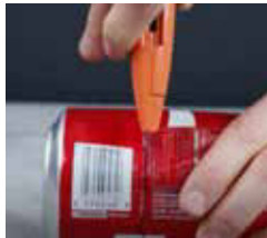
Cut off bottom of can with a craft knife
