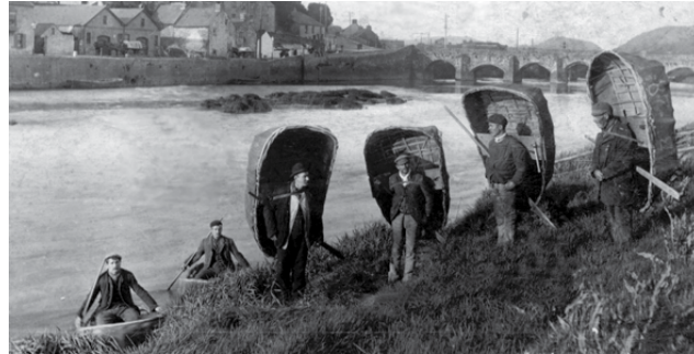
The picture shows traditional Welsh coracle circa 1890. This craft is built using ash lathes and covered with cowhide.
