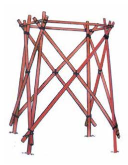
Ten minute tower can be build using light pioneering poles, scout staves or thick 30 mm bamboo staves (not garden bamboo sticks) to achieve 10 minute objective. It is not possible to build the tower in 10 minutes using heavy pioneering poles.
