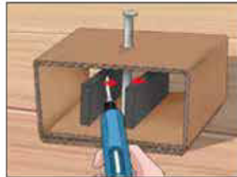
Glue magnets to nail
