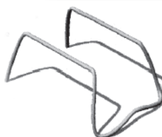
Step 4 Make 6-8 vertical cuts around the top. Make the cuts up to but not over the rounded edge. Slowly press the top into the bottom. ( a small board can help to make this easier)
