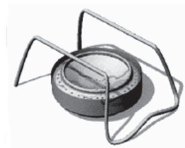
Step 2 Drill a number of holes (18-30) around the edge of the top and in the center as shown using a 2mm drill bit.
